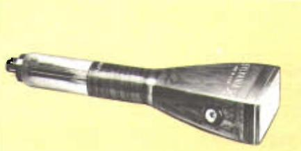
operating temperatures and low drain from battery or flyback heater supplies. Advanced powder metallurgy processes make possible a flat, pancake-like heater-cathode assembly, only .050" in diameter and .011" thick. Extreme low mass minimizes the possibility of damage from vibration and shock. It is adaptable to practically all present CRT designs.
